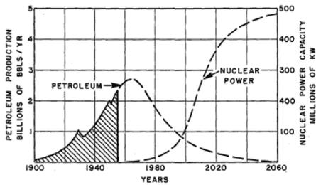
Figure 29 - Concurrent declines of petroleum production and rise of production of nuclear power in the United States. Growth rate of 10 percent per year for nuclear power is assumed; actual rate may be twice this amount.
